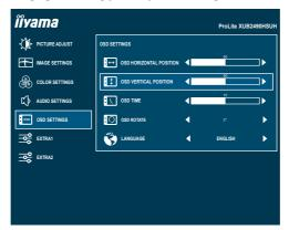
When you press the INPUT Button to end the adjustment, all changes are saved in the memory.
